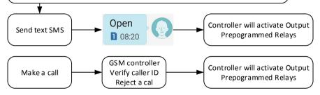
3. To Remote control GSM communicator Outputs Relays please , send the following SMS message from user phone number.
